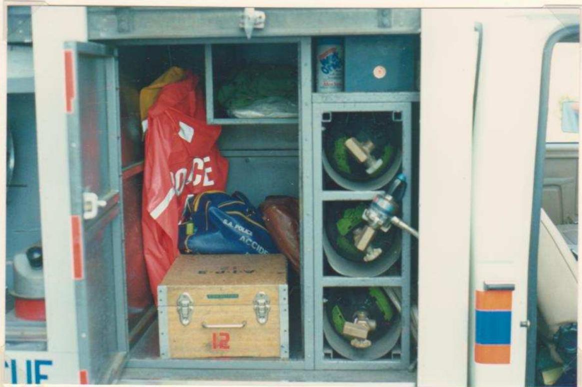
Portable Air. For use on air bags and air chisels (seldom used).
